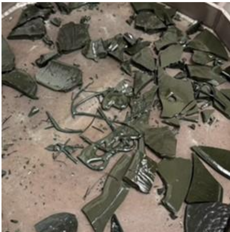
Figure B.38. Photographs of HS24-38 after the second melt using a tilt-pour furnace.
