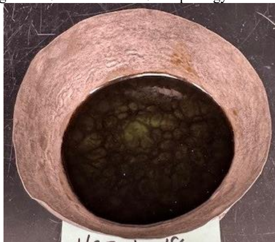
Figure E.18. Glass HS24-18 morphology after CCC.
