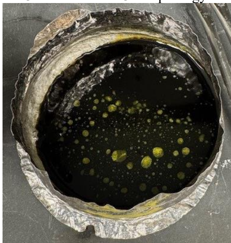
Figure E.24. Glass HS24-24 morphology after CCC.
