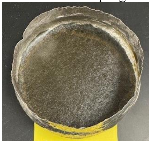
Figure E.30. Glass HS24-30 morphology after CCC.
