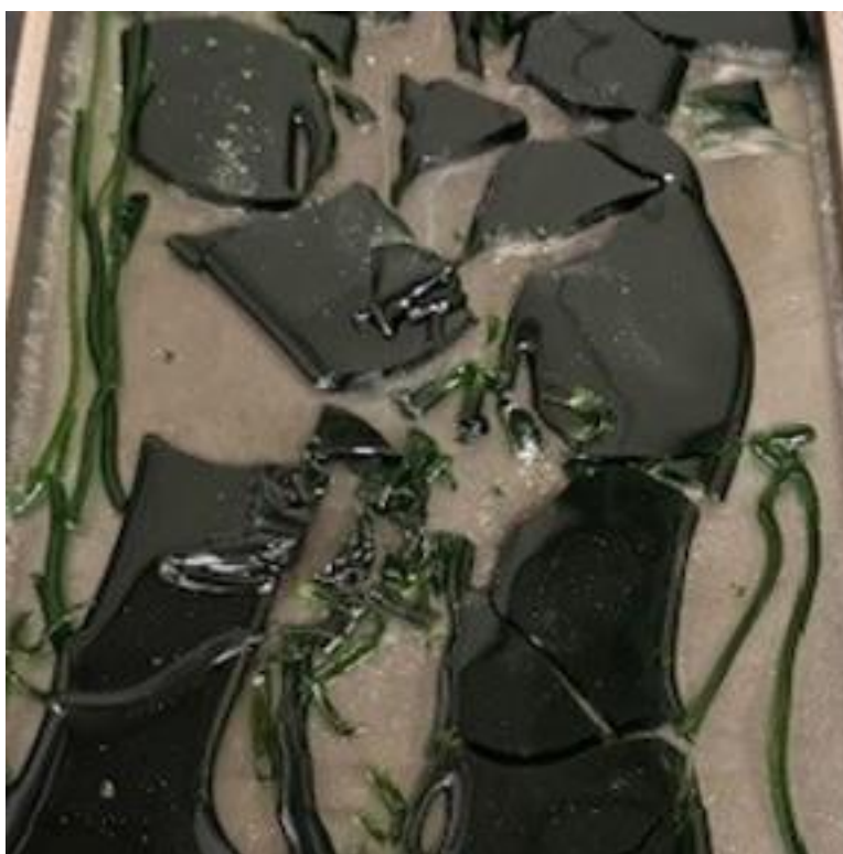
Figure B.49. Photographs of HS24-49 after the second melt using a Deltech furnace.
