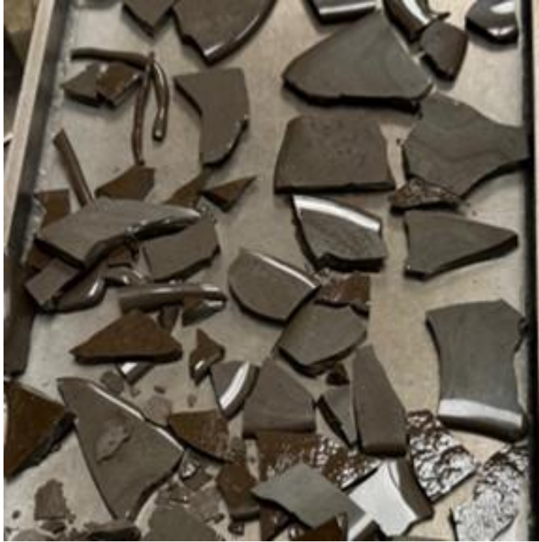
Figure B.12. Photographs of HS24-12 after the second melt using a Deltech furnace.
