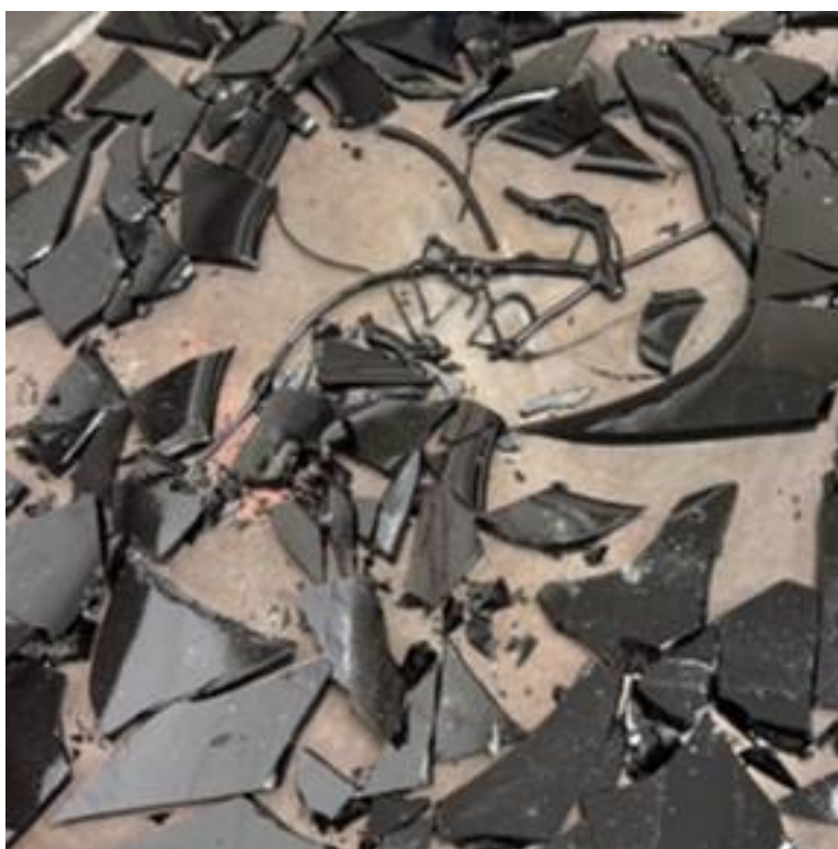
Figure B.31. Photographs of HS24-31 after the first melt using a tilt-pour furnace.
