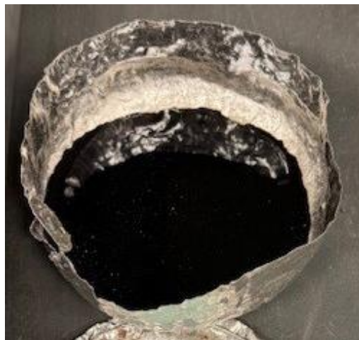
Figure E.19. Glass HS24-19 morphology after CCC.
