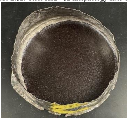
Figure E.33. Glass HS24-33 morphology after CCC.
