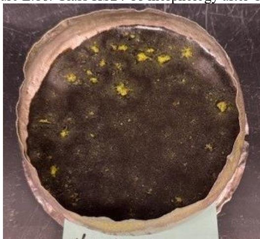
Figure E.17. Glass HS24-17 morphology after CCC.
