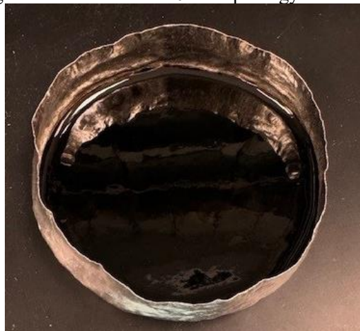
Figure E.2. Glass HS24-02 morphology after CCC.
