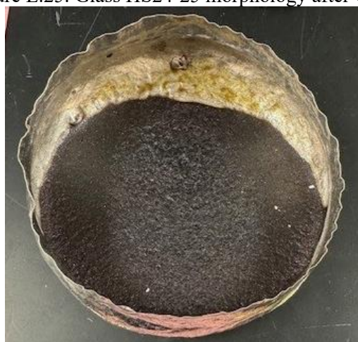
Figure E.26. Glass HS24-26 morphology after CCC.
