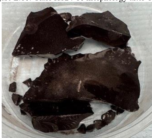
Figure E.11. Glass HS24-11 morphology after CCC.
