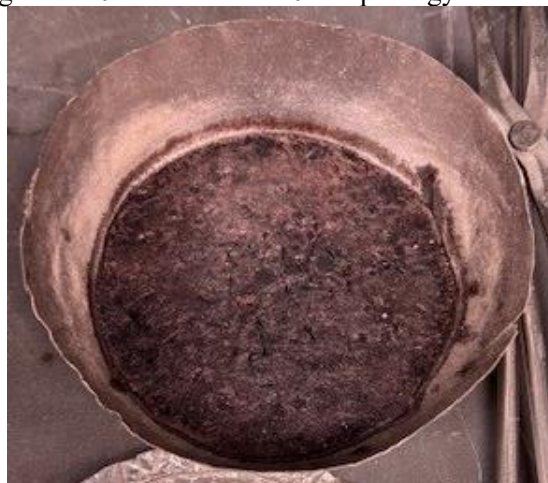
Figure E.21. Glass HS24-21 morphology after CCC.
