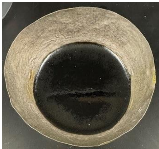
Figure E.31. Glass HS24-31 morphology after CCC.
