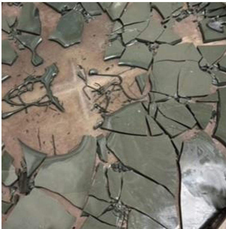
Figure B.34. Photographs of HS24-34 after the second melt using a tilt-pour furnace.
