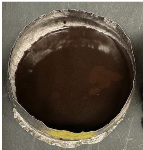
Figure E.22. Glass HS24-22 morphology after CCC.
