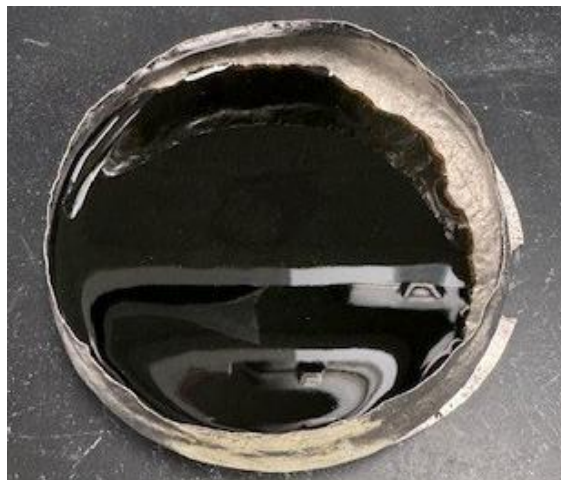
Figure E.40. Glass HS24-40 morphology after CCC.
