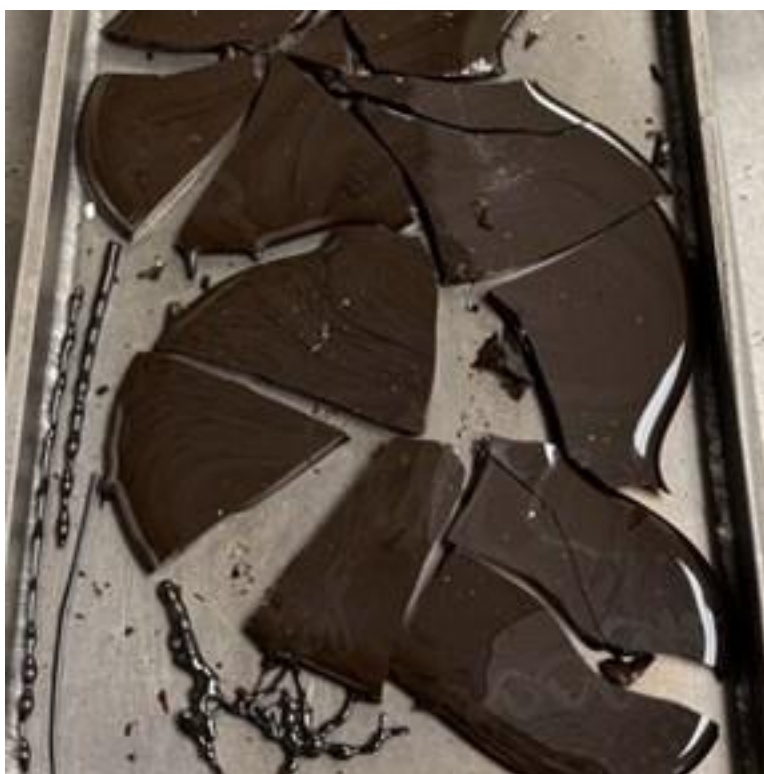
Figure B.45. Photographs of HS24-45 after the second melt using a Deltech furnace.
