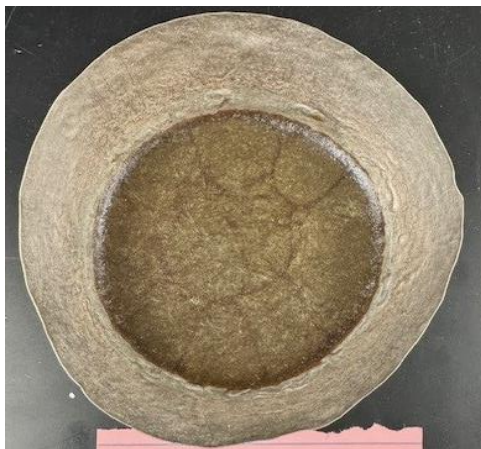
Figure E.25. Glass HS24-25 morphology after CCC.
