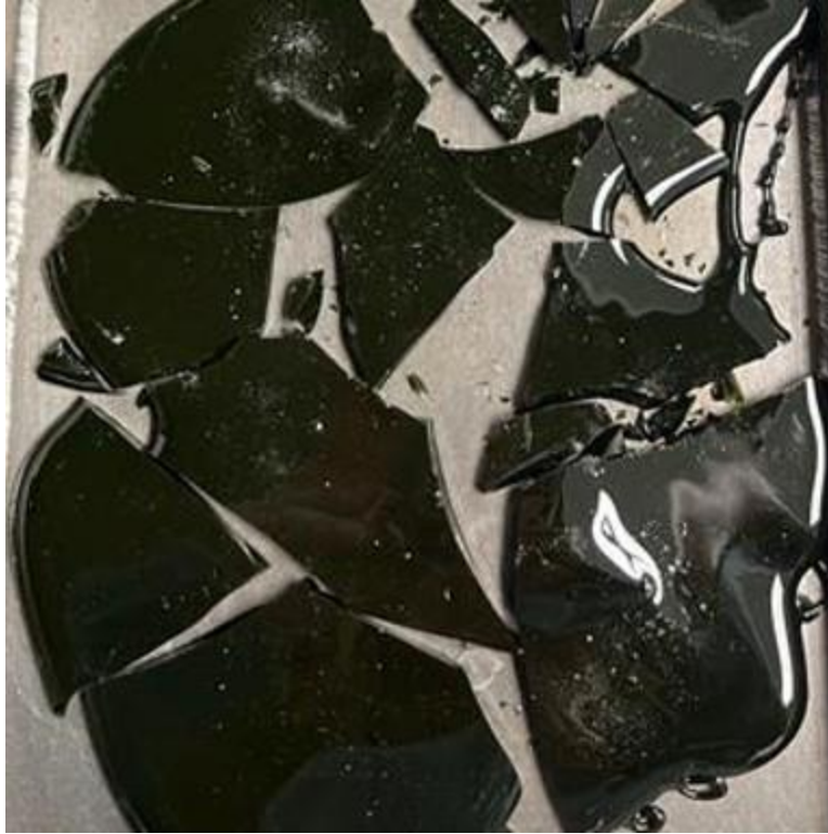
Figure B.32. Photographs of HS24-32 after the first melt using a Deltech furnace.
