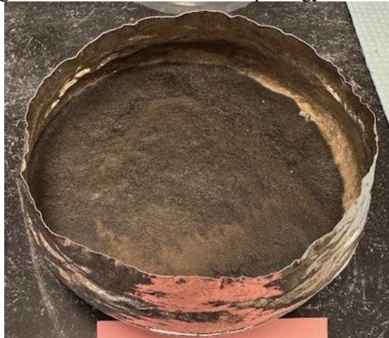
Figure E.39. Glass HS24-39 morphology after CCC.
