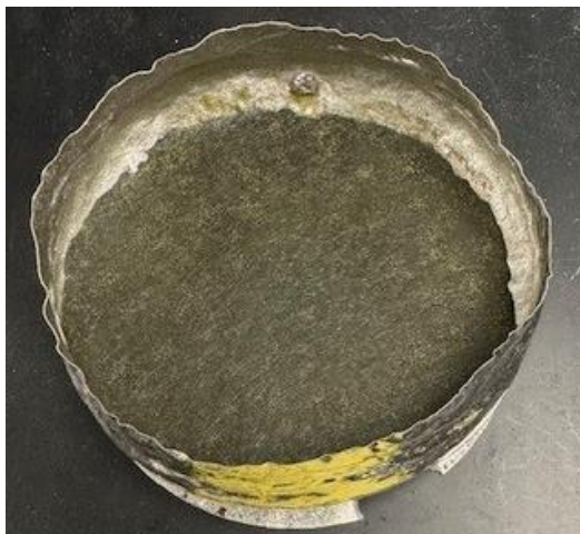
Figure E.34. Glass HS24-34 morphology after CCC.
