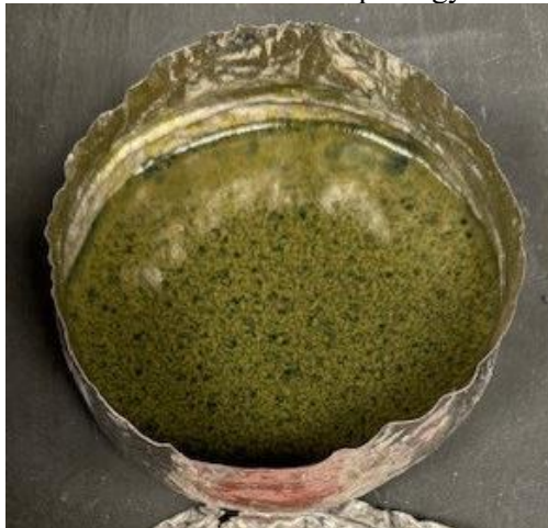
Figure E.6. Glass HS24-06 morphology after CCC.
