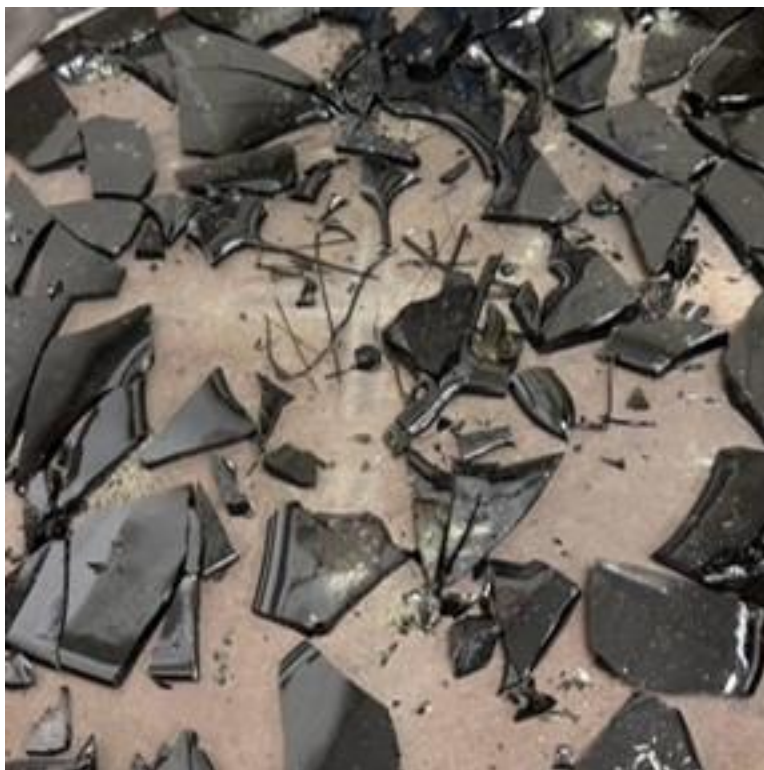
Figure B.36. Photographs of HS24-36 after the first melt using a tilt-pour furnace.
