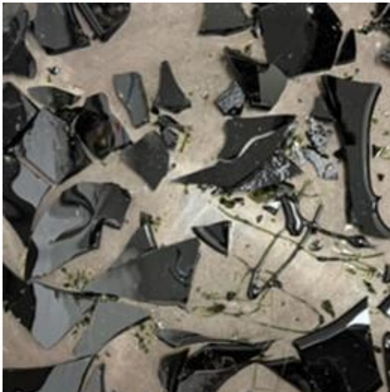
Figure B.1. Photographs of HS24-01 after the first melt using a tilt-pour furnace.
