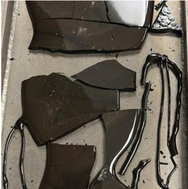
Figure B.46. Photographs of HS24-46 after the second melt using a Deltech furnace.
