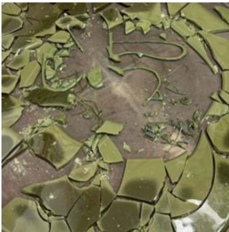
Figure B.27. Photographs of HS24-27 after the first melt using a tilt-pour furnace.
