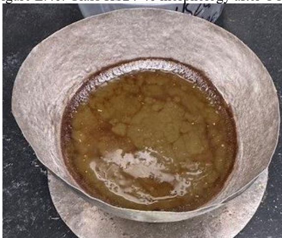
Figure E.41. Glass HS24-41 morphology after CCC.
