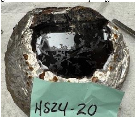
Figure E.20. Glass HS24-20 morphology after CCC.
