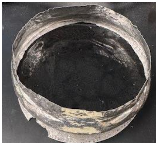
Figure E.43. Glass HS24-43 morphology after CCC.
