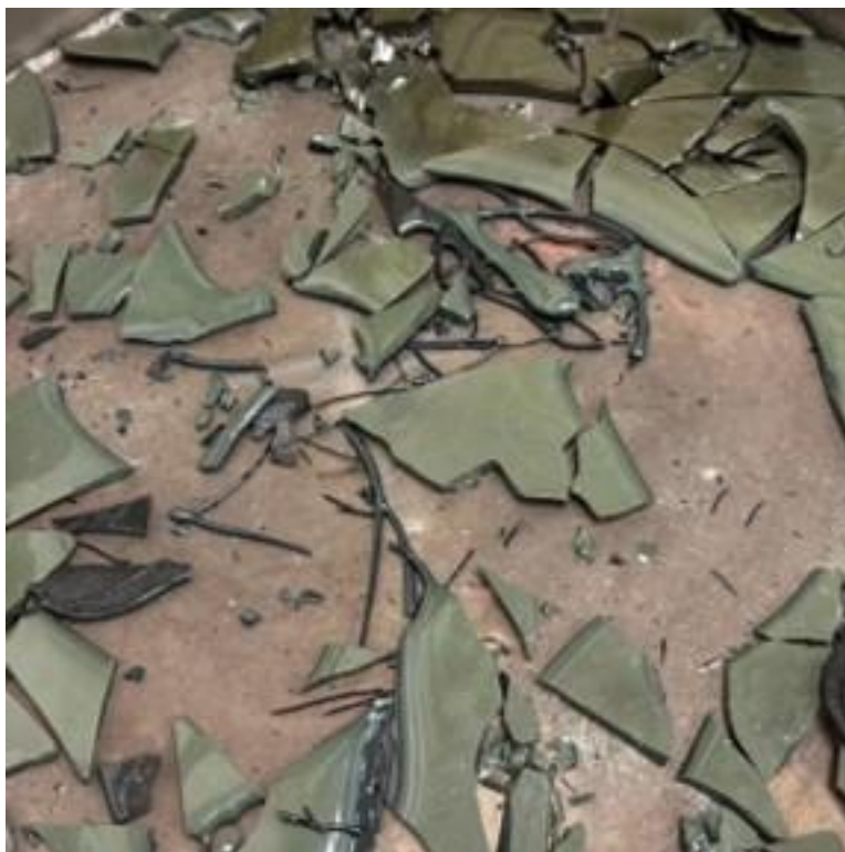
Figure B.30. Photographs of HS24-30 after the first melt using a tilt-pour furnace.
