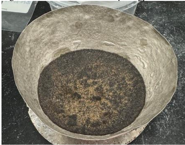
Figure E.38. Glass HS24-38 morphology after CCC.
