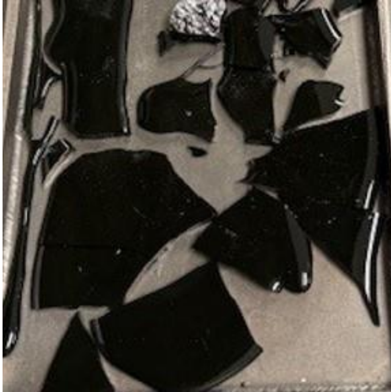
Figure B.50. Photographs of HS24-50 after the second melt using a Deltech furnace.
