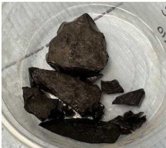
Figure E.10. Glass HS24-10 morphology after CCC.
