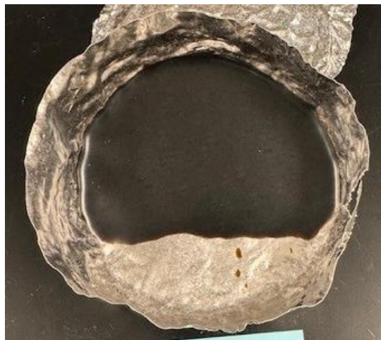
Figure E.4. Glass HS24-04 morphology after CCC.
