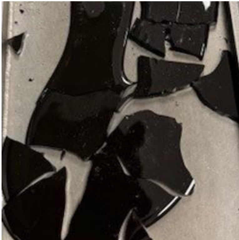
Figure B.19. Photographs of HS24-19 after the second melt using a Deltech furnace.
