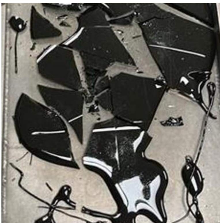
Figure B.35. Photographs of HS24-35 after the second melt using a Deltech furnace.
