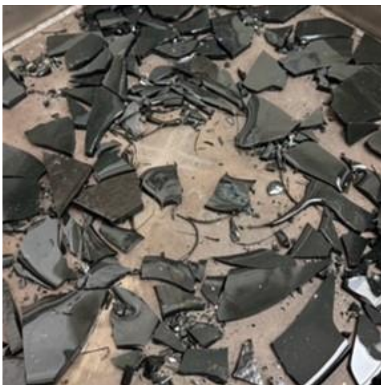
Figure B.39. Photographs of HS24-39 after the second melt using a tilt-pour furnace.
