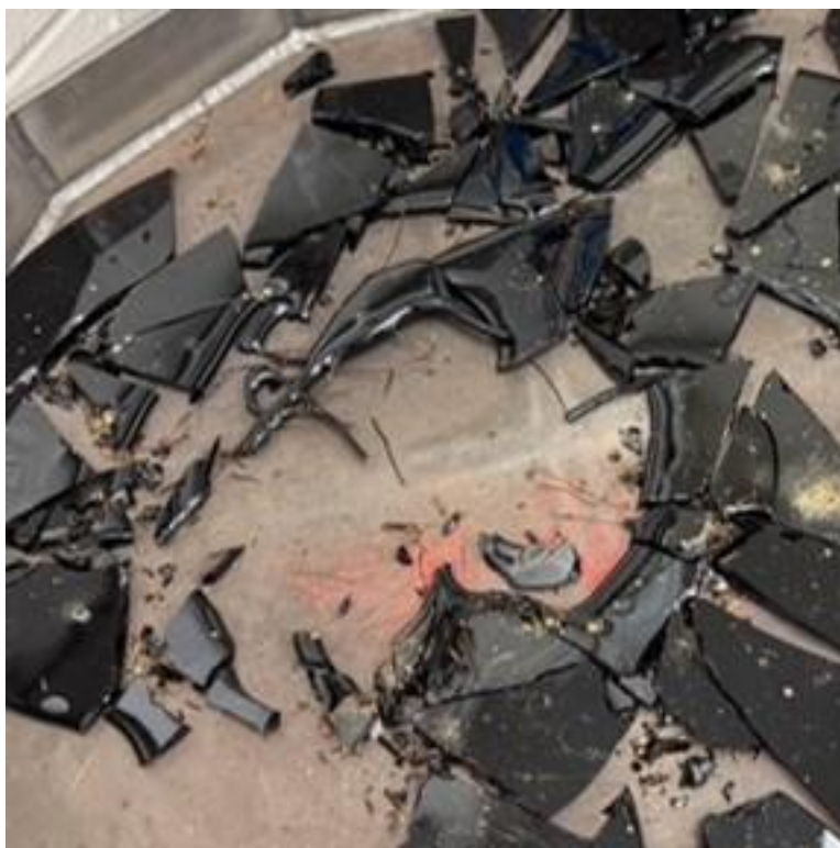
Figure B.37. Photographs of HS24-37 after the first melt using a tilt-pour furnace.
