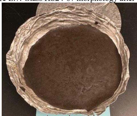
Figure E.8. Glass HS24-08 morphology after CCC.
