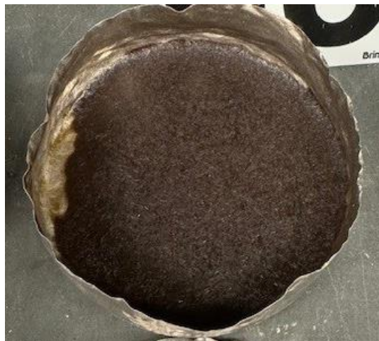
Figure E.7. Glass HS24-07 morphology after CCC.
