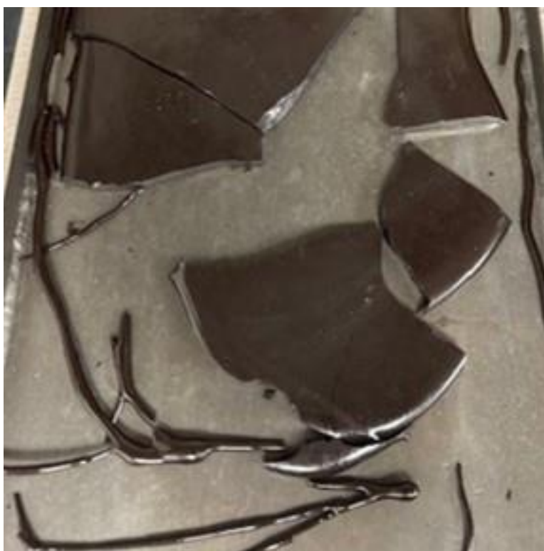
Figure B.23. Photographs of HS24-23 after the second melt using a Deltech furnace.
