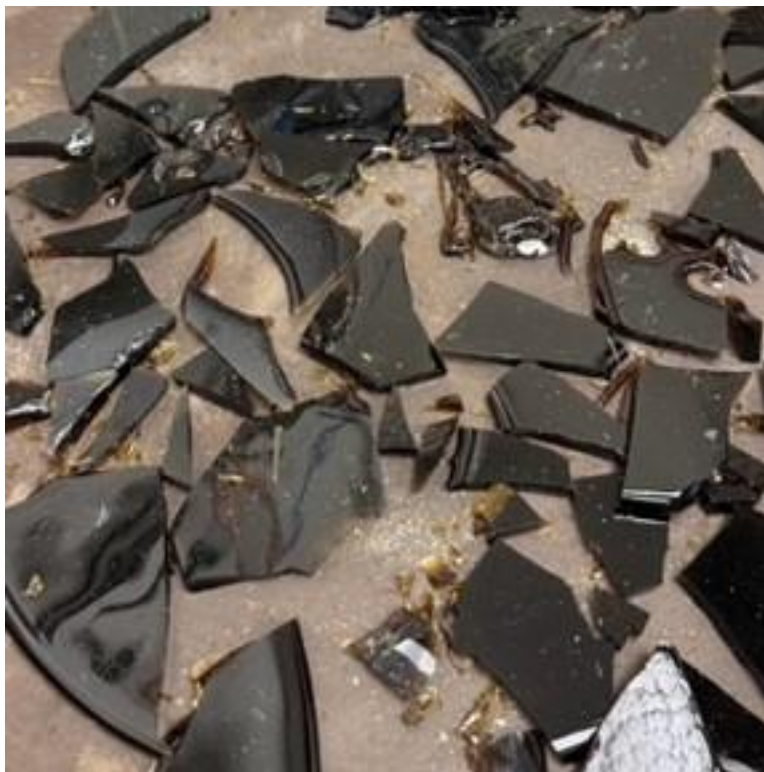
Figure B.41. Photographs of HS24-41 after the second melt using a tilt-pour furnace.
