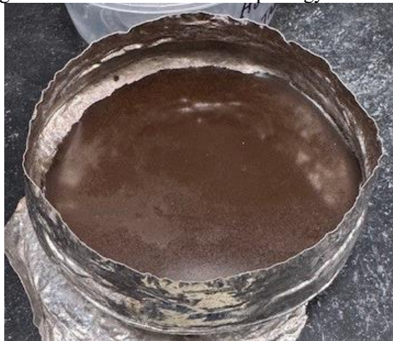
Figure E.42. Glass HS24-42 morphology after CCC.
