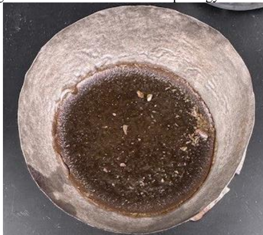
Figure E.47. Glass HS24-47 morphology after CCC.
