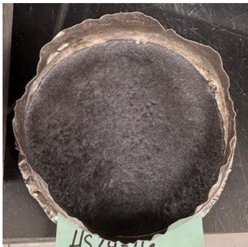
Figure E.16. Glass HS24-16 morphology after CCC.
