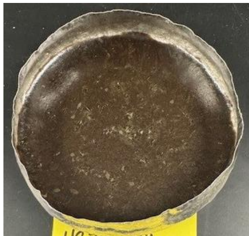
Figure E.28. Glass HS24-28 morphology after CCC.
