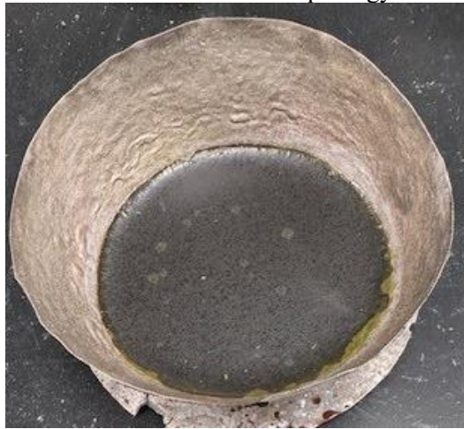
Figure E.50. Glass HS24-50 morphology after CCC.
