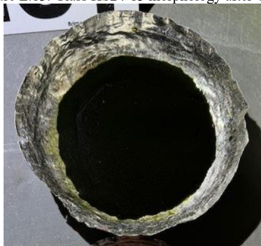
Figure E.14. Glass HS24-14 morphology after CCC.
