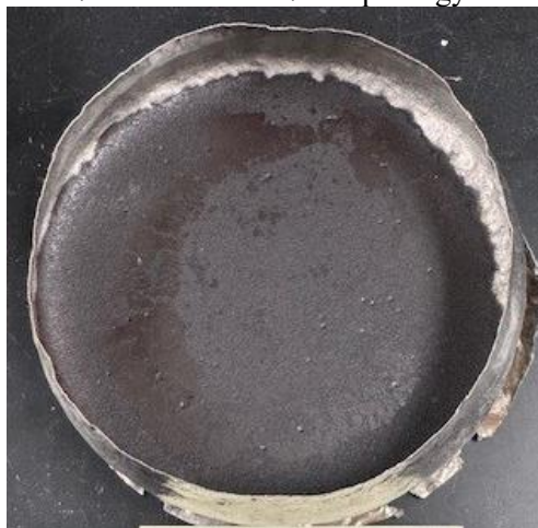
Figure E.48. Glass HS24-48 morphology after CCC.
