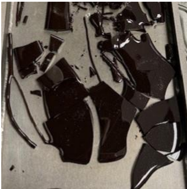
Figure B.26. Photographs of HS24-26 after the second melt using a Deltech furnace.
