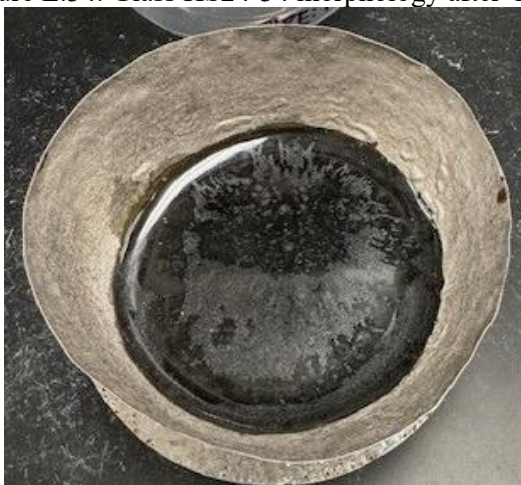
Figure E.35. Glass HS24-35 morphology after CCC.
