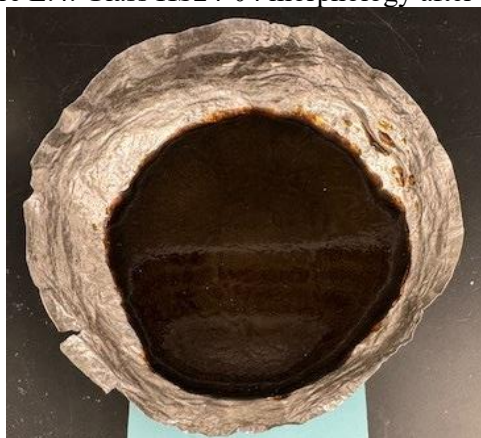
Figure E.5. Glass HS24-05 morphology after CCC.
