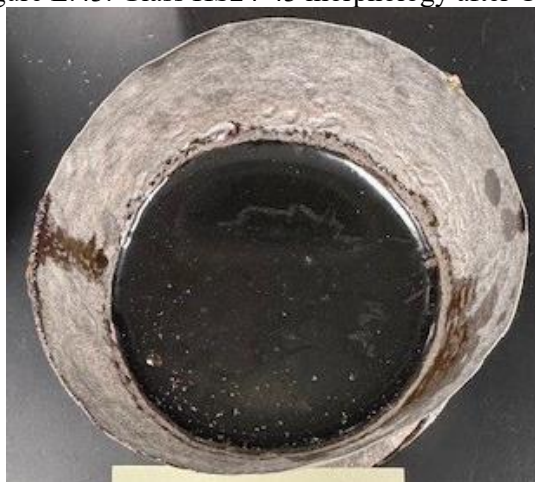
Figure E.44. Glass HS24-44 morphology after CCC.
