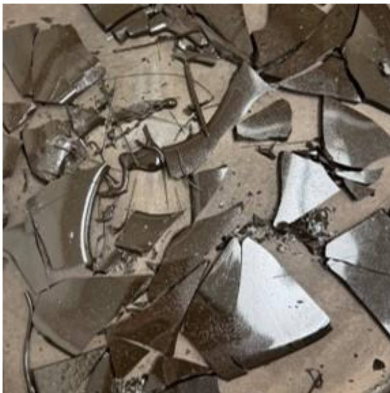
Figure B.8. Photographs of HS24-08 after the first melt using a tilt-pour furnace.
