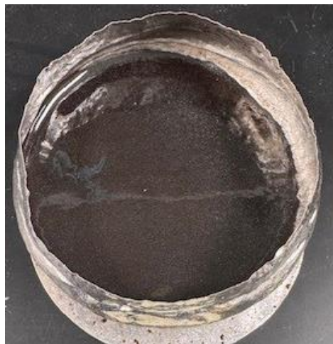
Figure E.46. Glass HS24-46 morphology after CCC.
