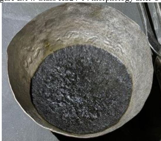
Figure E.15. Glass HS24-15 morphology after CCC.
