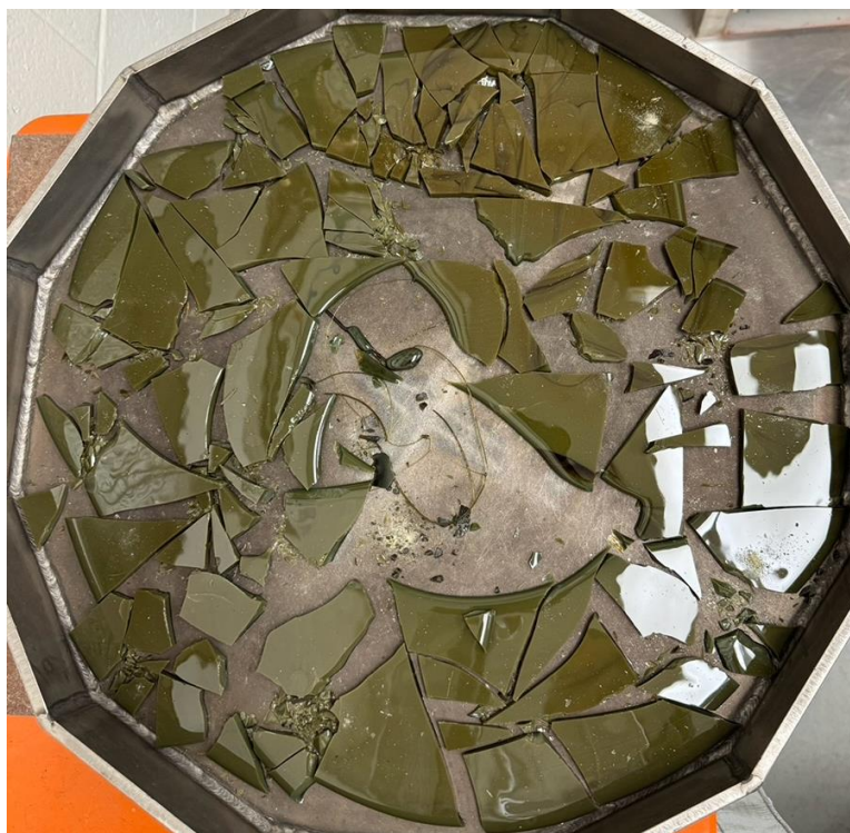
Figure B.5. Photographs of HS24-05 after the second melt using a tilt-pour furnace.
